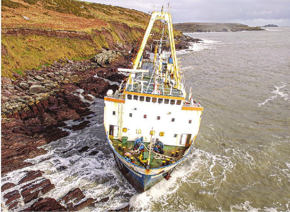
The MV Alta shortly after she ended up on the shore of Ballyandreen pictured by Brian Motyer in 2020. The ship has since deteriorated from sea conditions. The mid-section has broken away leaving the bow and stern separately wedged on the rocks.
